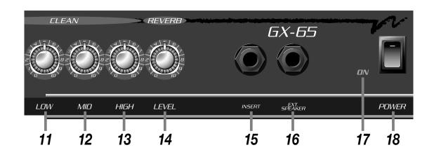
**15: INSERT:** Use this jack to connect an external effects device to the amplifier. Use a stereo 1/4" male Y-cord: ring = send, tip = return, sleeve = ground. See the illustration to the right for more information.
